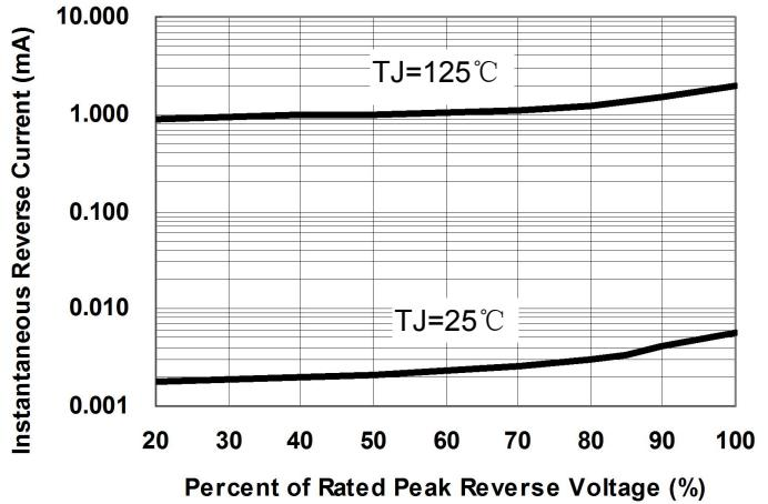
Fig.2-Typical Reverse Current
