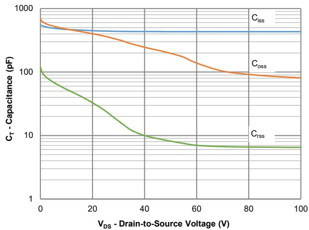
Figure 9: Capacitance Characteristics
