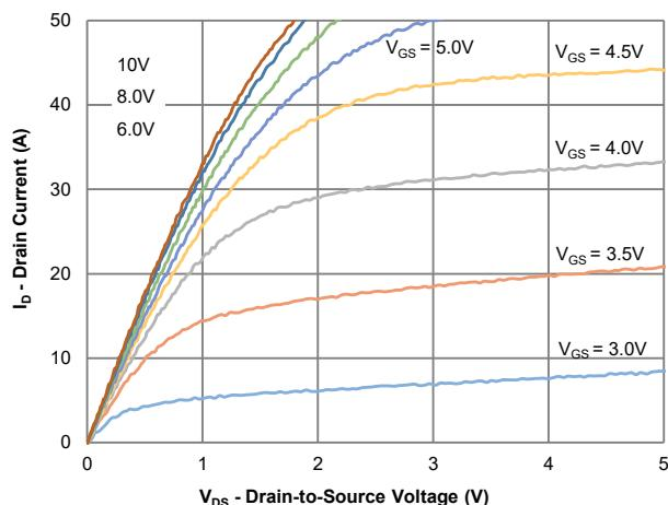
**Figure 1: Output Characteristics**
