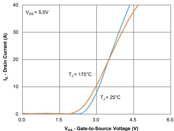
**Figure 2: Transfer Characteristics**
