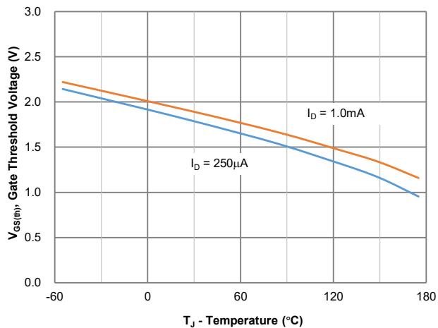
Figure 7: Gate Threshold Variation vs. Junction Temperature
